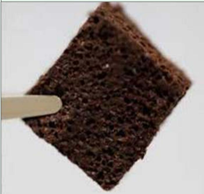
A foam filter made with used coffee grounds removes lead and mercury from contaminated water.
