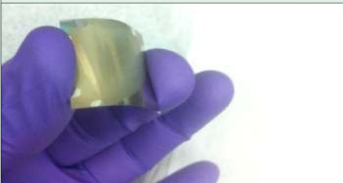
Ohio State University researchers have developed a technique to create light emitting diodes on metal foil
