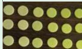
Paper matrices with entrapped bacteria and colouring showing samples of different toxicity levels
